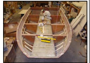
9m Test boat during fit out
