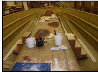
New 11m during moulding
